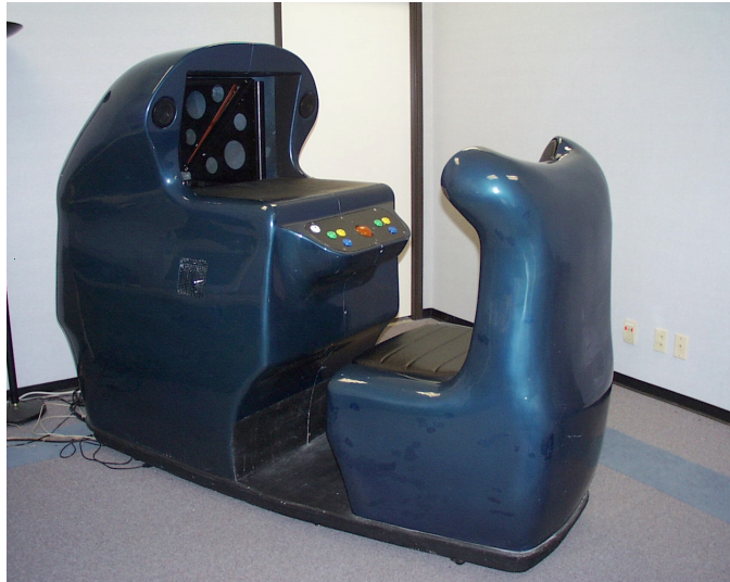
Figure 3: Previous 25"-screen prototype incased in an arcade-game-style shell.
