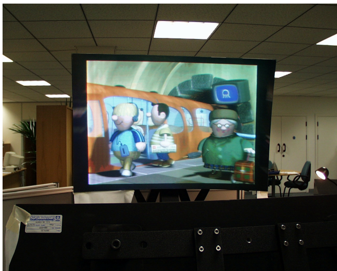
Figure 7: Actual image on the 50" display screen showing how the picture-shape correction on the raster scan gives a rectilinear image.
