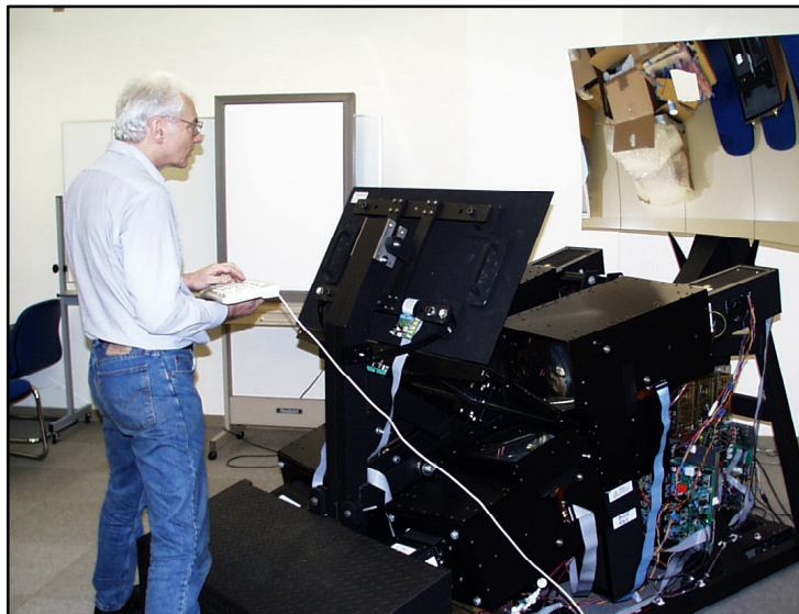
Figure 8: Adjustments are made to the picture shape by software control on the 50" display for a demonstration in Japan.
