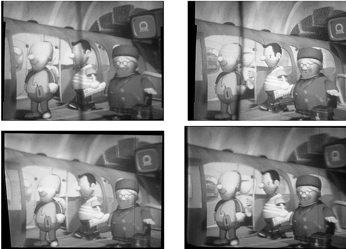
**Figure 6:** Photographs of the display with and without the lenticular diffuser. The dark line in each of the upper images (no lenticular diffuser) is caused by the join between two optical systems. The lenticular diffuser removes this effect without detriment to image quality.
