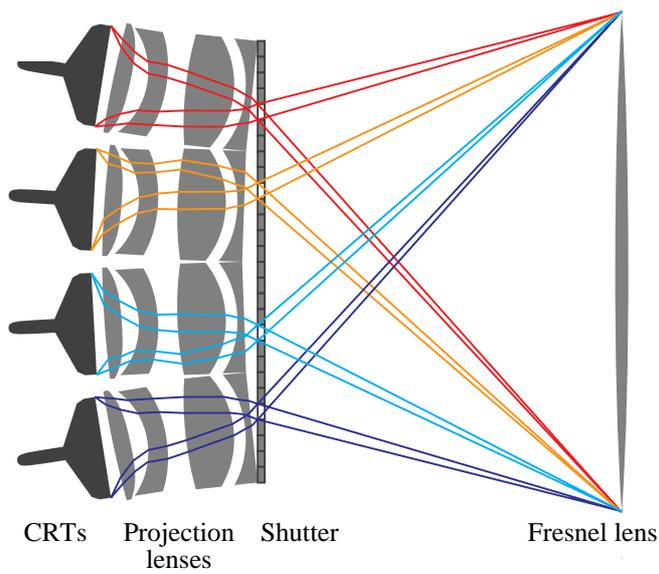
**Figure 3:** The new 28 view, multi-projector, time sequential display. Multiple CRTs and their associated projection lenses are placed behind a single shutter. The front elements of the lenses abut. Note that the compound lenses in this figure are indicative only; they are not exact representations.
