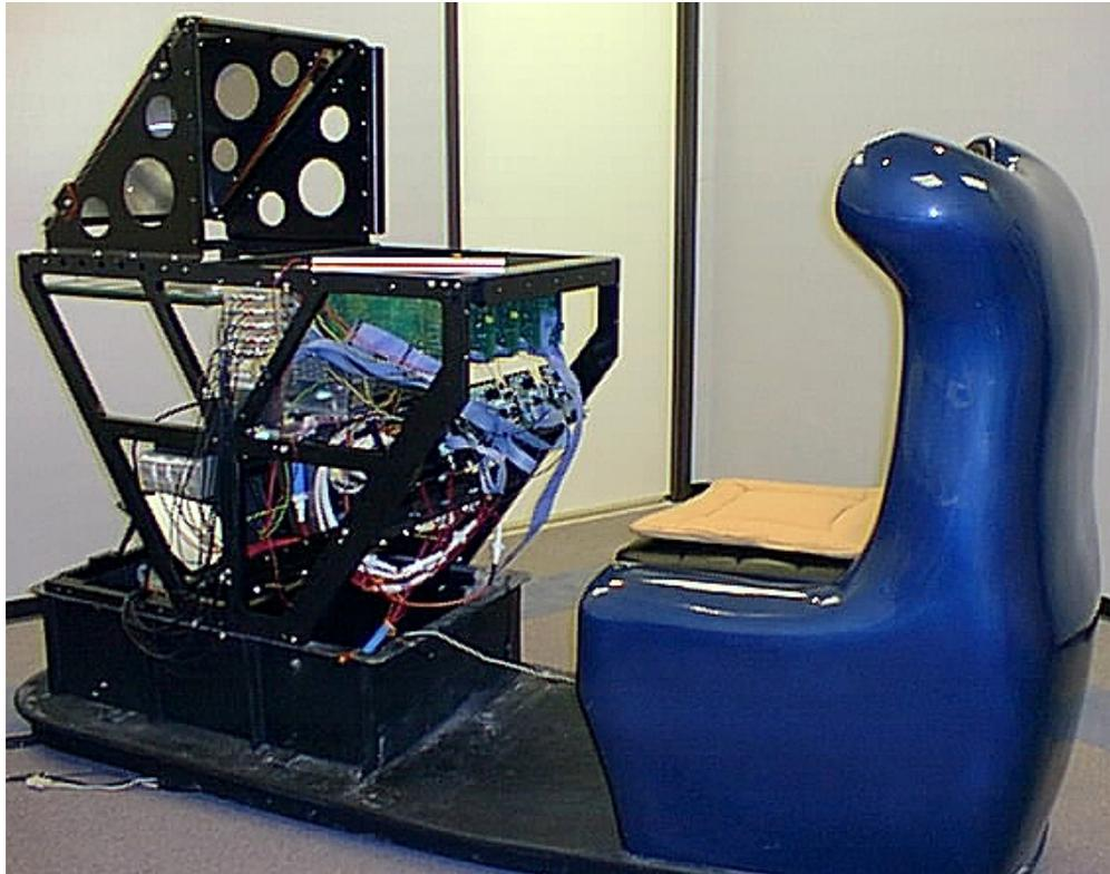
**Figure 5:** The completed display. The viewer sits in the large chair and views the horizontally mounted Fresnel lens via the diagonally mounted plane mirror. Beneath the Fresnel lens is a second plane mirror. The CRTs and projection lenses are mounted in the right hand half of the housing.
