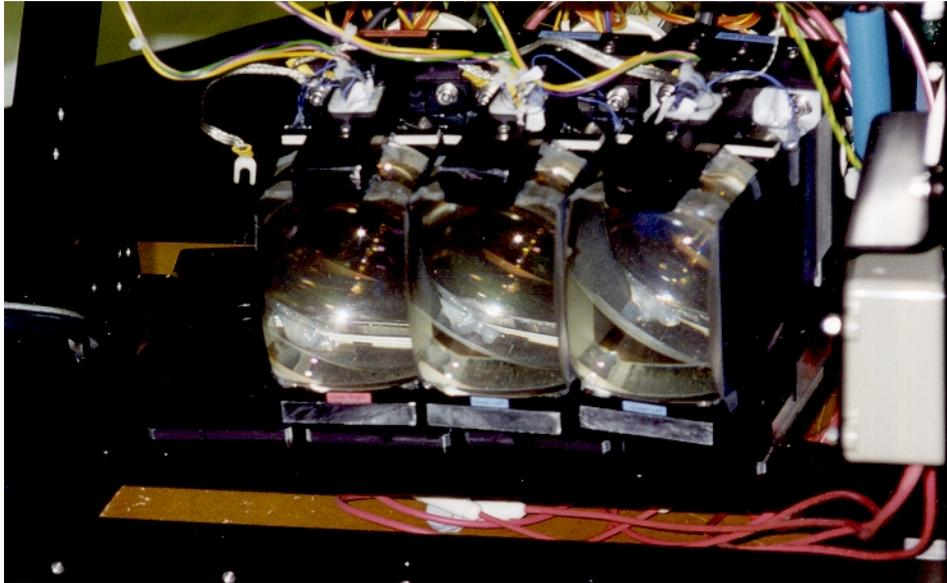
**Figure 4:** The display under construction. This picture shows the front elements of three of the four projection lenses. The fourth will be placed in the space at left and the shutter then placed in front of all four.
