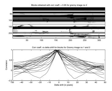
Figure 11. Outcome of row decomposition algorithm, showing blocks in black obtained using 0.95 correlation threshold and the corresponding block correlation coefficient. The maximum correlation lies within the [-4 4] pixel range.
