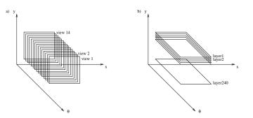
Figure 4. Two different possibilities of scanning the x, y and  $\theta$  dimensions: a) view by view b) layer by layer.
