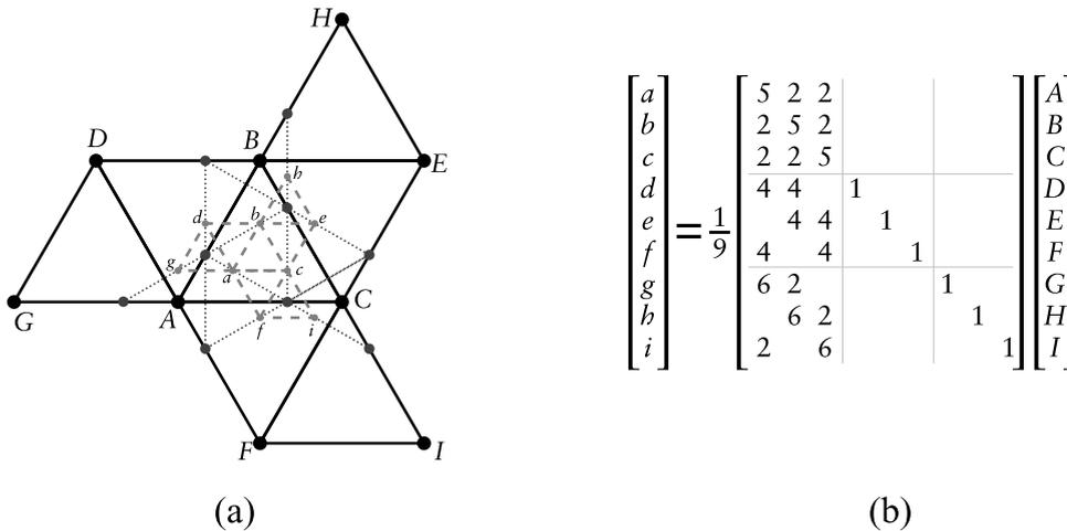
**Fig. 6.** Eigenanalysis: (a) the self-similar region after two steps of subdivision. (b) the associated matrix.
